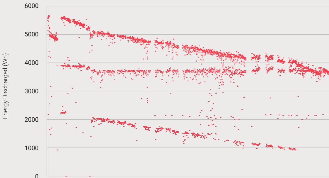
Figure 4. Energy discharged per cycle by the Tesla Powerwall 1 battery pack
