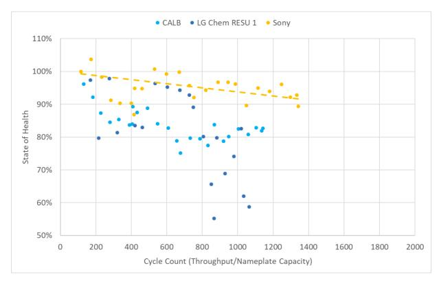
Figure 3 Average capacity fade results for Phase 1 Batteries
