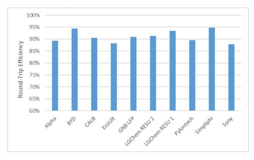
Figure 5. Average round-trip efficiency of various battery packs
