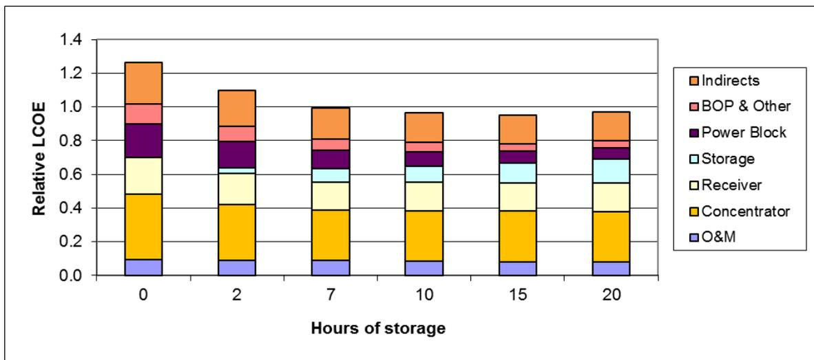
Figure C3: Modelling LCOE as a function of storage hours for a molten salt tower plant for Longreach Qld<sup>34</sup>.
