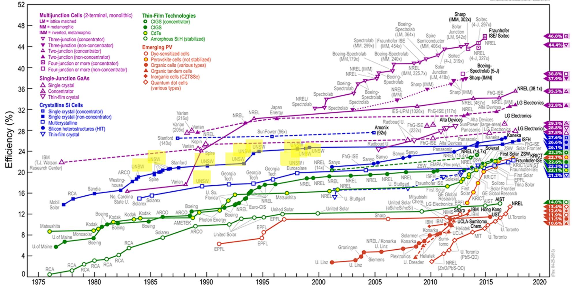
Figure 15: PV Cell types and efficiencies over time (NREL, 2018)<sup>12</sup>
