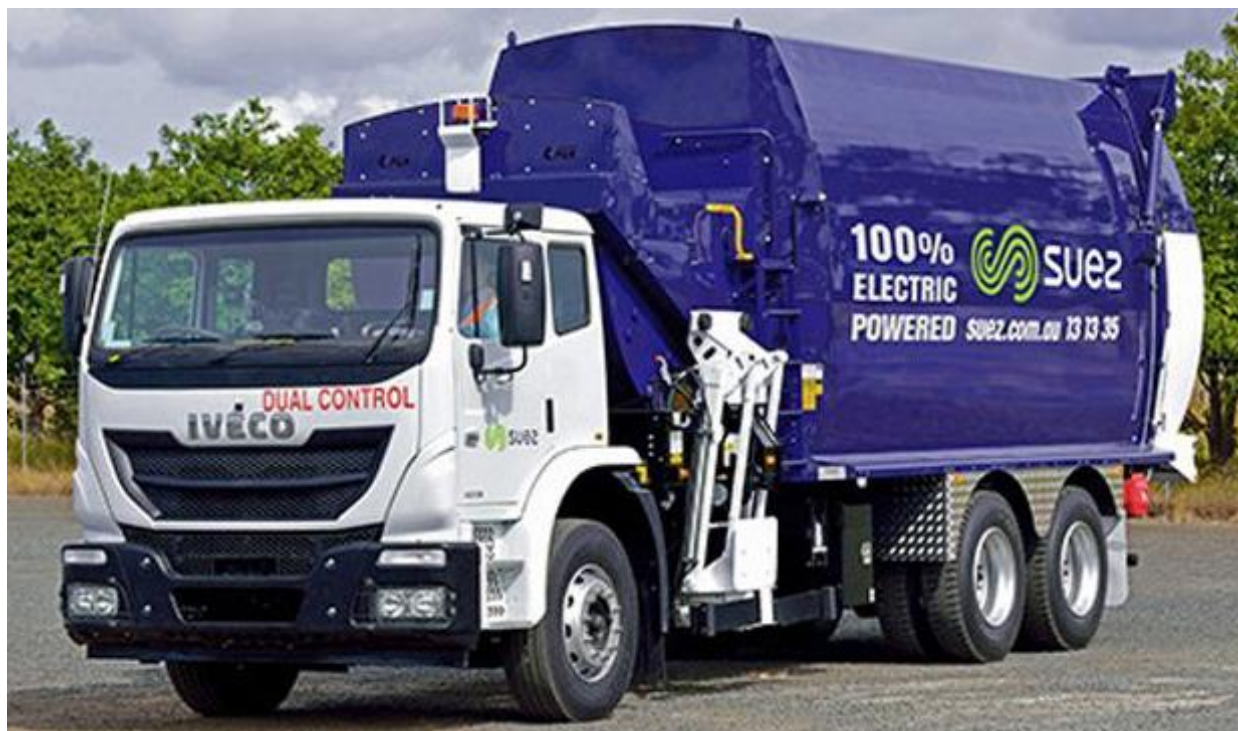
Figure 29 An example of one of SEA Electric's rubbish trucks, with up to 230 km driving range
