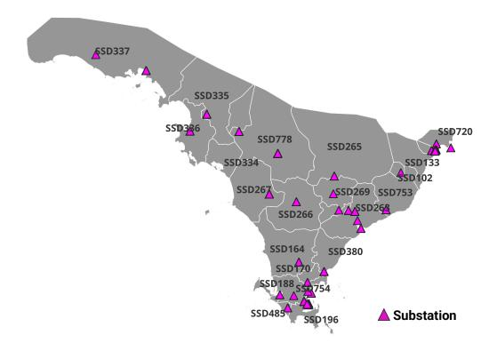
The SAPN distribution network in the Eyre Peninsula is partitioned into 28 zone-substations (ZS) labelled by a unique substation district (SSD) identification number. Each zone has one or more substation junctions which act as a distribution point to all assets within that zone. Substations that supply a particular zone are typically found within that zone, however, there are exceptions such as SSD334.
