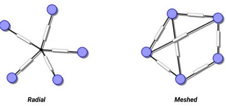
Figure 35: Meshed and radial network topology
