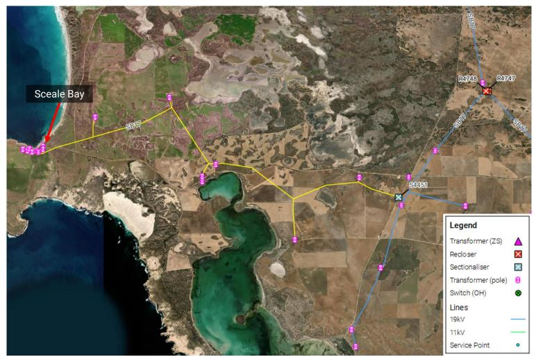
Figure 33: Proposed extent of the intermittent microgrid for Sceale Bay (yellow)
