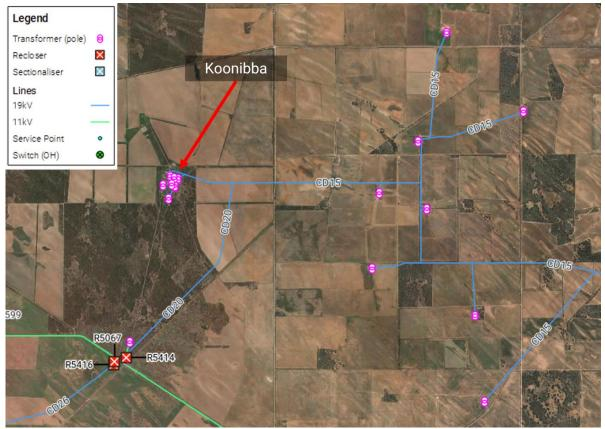
Figure 6: Feeder CD20 supplying Koonibba
